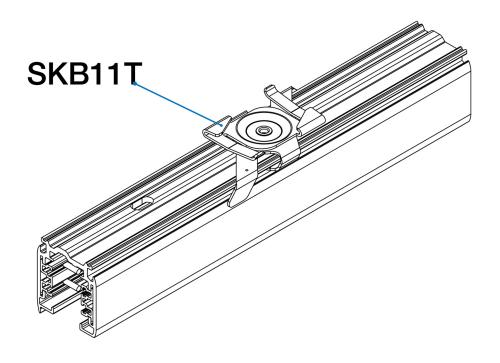
Fmax 50N / Track clip only, T-bar according to the manufacturer. Recommended distance between clips 750mm
