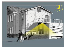
② With insufficient ambient light, the sensor switches on the light when motion is detected.
